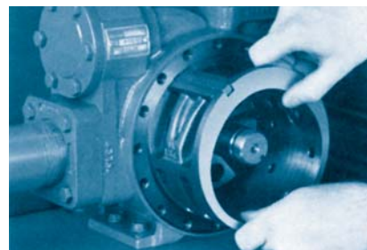
Easily replaceable liner restores efficiency.
