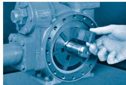
Simple vane replacement requires no special tools.
